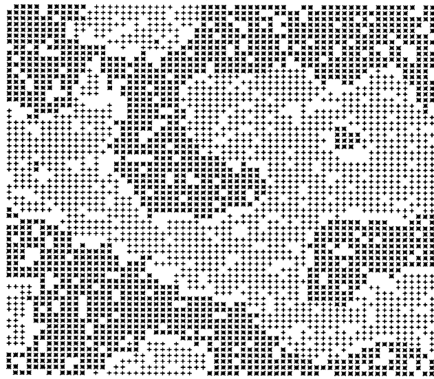
FIG. 2. A two-dimensional cross section (planar view) of a realization of the Monte Carlo model at t = 100\,000 MCM. The domains of A(+) and B(*) are quite distinct and interpenetrating. Note that the vacancies are often found at interface but are also found inside domains.
